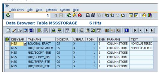
The output is already filtered. It only contains rows that belong to the column-store configuration (PARNAME = "COLUMNSTORE"). If there is no single configuration regarding the column-store in table MSSSTORAGE yet, the Data Browser does not start. Instead, the following status message appears:
