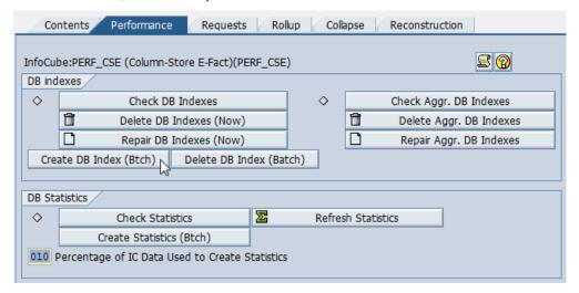
There are two buttons that both start a batch job for the index repair:
